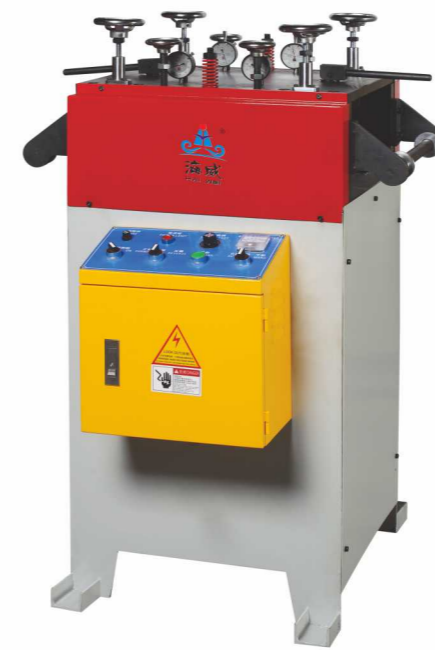
BCL 整平厚度Material thickness range: 0.3-1.5mm
